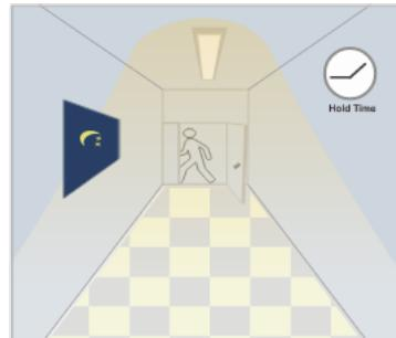
After hold time, the sensor dims the lamp at a low light level if no new motion trigger.
